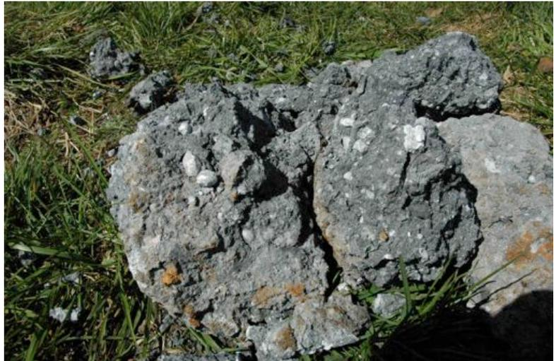
Salt slag showing lumps of recoverable aluminium
